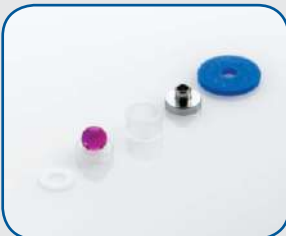
MODEL: M6KA, 510, 515, 600, 610, LC MODULE 1 CTS-0110 KIT OEM WAT060495 Inlet Check Valve Rebuild Kit rebuilds 2 valves • Blue Washer (CTS-0101) 2 • Gasket, Retainer (CTS-0102) 2 • Insert, PCTFE (CTS-0103) 2 • Check Ball & Seat 0125" (CTS-0104) 2 • Washer, PTFE (CTS-0105) 2
